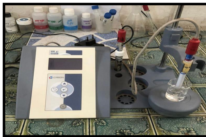
Figure 1 (Ion selective electrode (ISE).)
